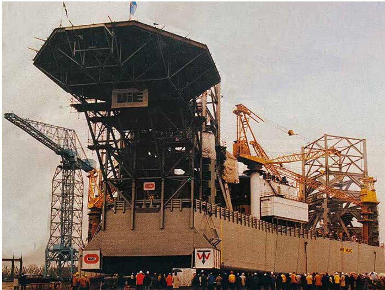
The 17 500t Transworld Gorilla class jackup launched at UIE's clydebank yard. It was then towed out under the Erskine bridge for the final installation of its 160m legs.
