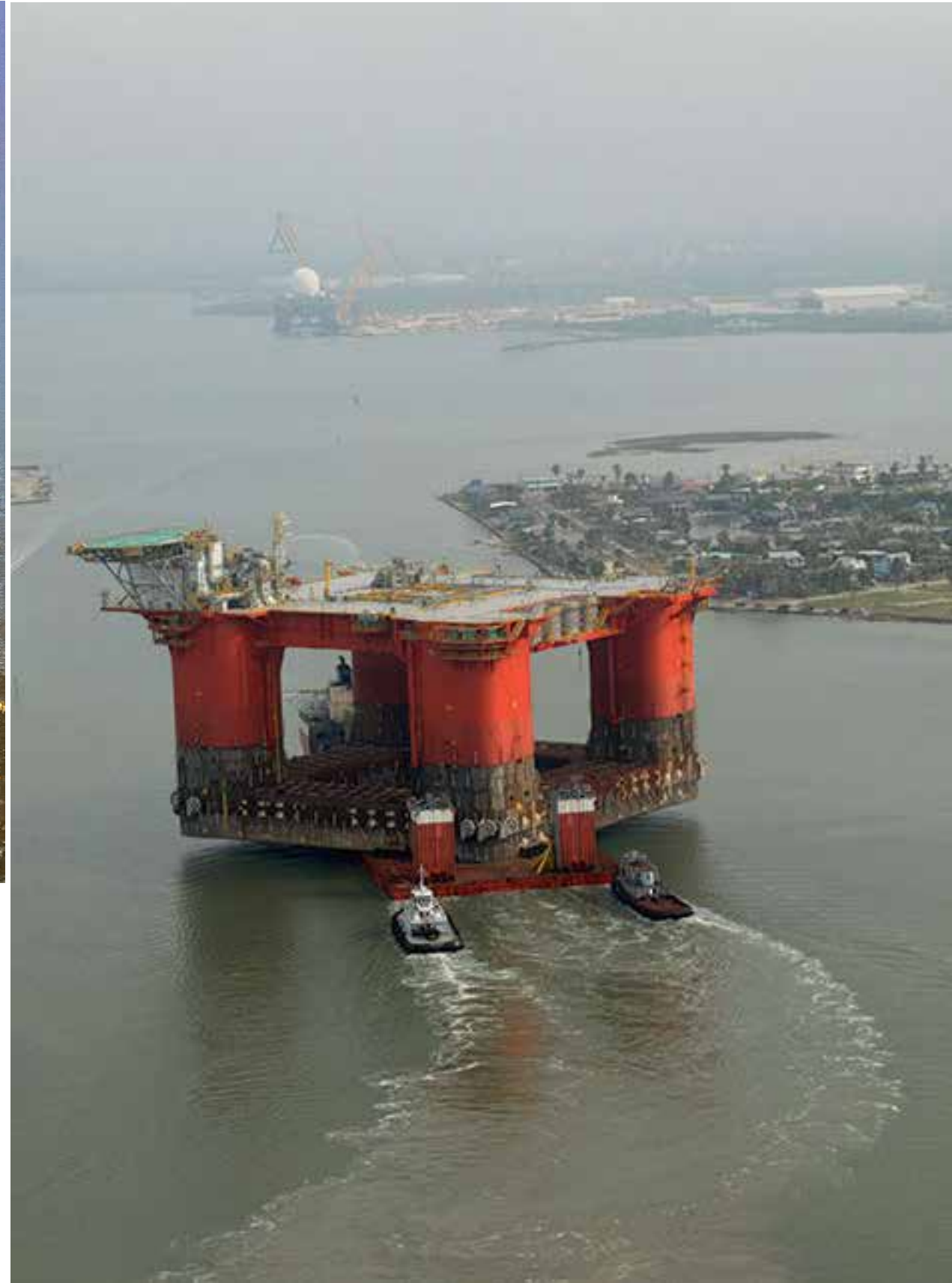
The hull leaving a Korean shipyard on a submersible transport vessel Check out what I think is the Odyssey in the background.
