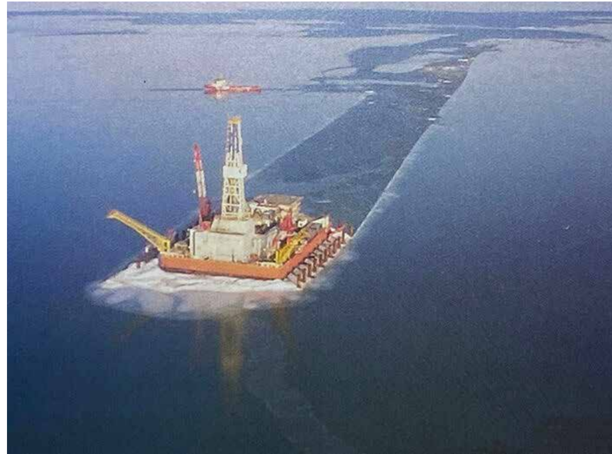
Friday Photos. Rig 257 in The Caspian Sea Drilling in shallow waters has its own difficulties but adding occasional sea ice makes it even more challenging. The Parker Rig 257 was converted from a drilling barge in Nigeria to an ice-resistant grounded barge
